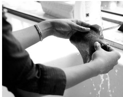
Gambar 6.8 Cara mencuci filter debu kipas alat TCM
